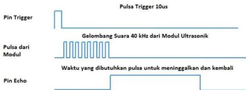
**Gambar 2. Timing diagram**
